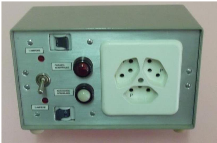
Figure 1 The finished appliance. On the left the switches of the both overcurrent releases: above "1A", below "2A".
