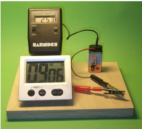
Figure 21 - Test set-up to measure the time dependent temperature increase of shorted out batteries.
