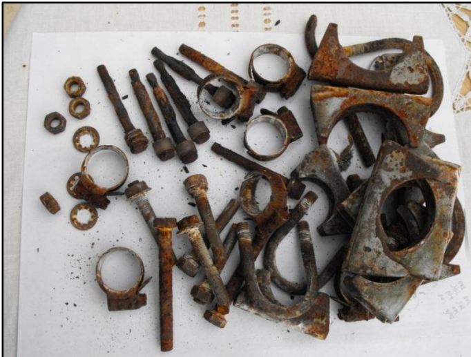
The condition of some of the clamp and bolts that were removed.
