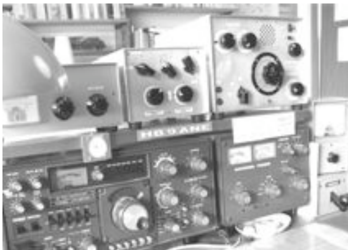
fig 1: My station with the home-made regenerative receiver 1-v-2 showing the new AT next to it.
