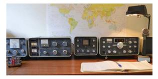
this time will be the KW2000D at the RSGB's National Radio Centre at Bletchley Park. It is one of that last KW2000s ever made, featuring a Nixie tube digital readout and was originally the company founder's personal radio. Fewer than five KW2000Ds were ever made; it is an extremely rare radio. As always, SSB/CW activity will be on any frequency ending in 77 ±QRM – 1.977, 3.777, 7.177, 14.177MHz etc. AM activity will be on VMARS frequencies.
