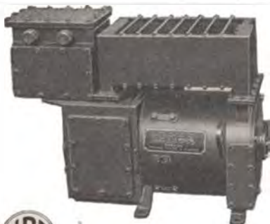
H.F. Motor Alternator for Radar. Output 2 KW. 80 volts A.C. 1,500 cycles per second. Watertight. Fitted with Automatic Voltage Regulator.
