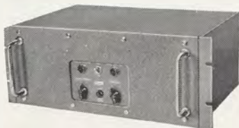
PR 71 Single channel crystal controlled V.H.F. receiver for R/T and M.C.W. in the 70-156 Mc/s band. High sensitivity and excellent stability over a wide temperature range. Local or remote control. The remote control unit incorporates a loudspeaker and provides all facilities, including automatic channel indication. Designed to International Aeradio Specification.
