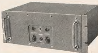
PR 71 Single channel crystal controlled V.H.F. receiver for R/T and M.C.W. in the 70-184 Mc/s band. High sensitivity and excellent stability over a wide temperature range. Local or remote control. The remote control unit incorporates a loudspeaker and provides all facilities, including automatic channel indication. Designed to International Aeradio Specification.
