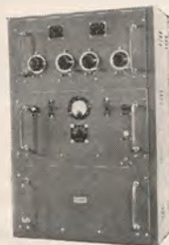
PT 15 50 watt V.H.F. transmitter covering the 118-132 Mc/s frequency range, but can be supplied for other frequency ranges between 70 and 184 Mc/s to order. The operational frequency is crystal controlled. Remote speech and "press to transmit" facilities over a distance of approximately 25 miles using a standard telephone pair.
