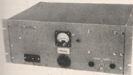
PV 14 Wide band aerial amplifier enabling up to ten communication receivers to be operated from one common aerial system. Handles large signal inputs without overloading or cross-talk becoming excessive. Low noise factor. Available for 75 or 600 ohm inputs. Designed to International Aeradio Specification.
