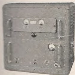
PT 10 12 watt V.H.F. crystal controlled transmitter covering the 116-132 Mc/s band. Designed for simple operation with band pass circuits in the R.F. unit to reduce the number of tuning controls required, and a pre-set circuit in the modulator which automatically prevents over modulation.
