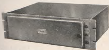
PR 51 H.F. Receiver for high quality reception of R/T M.C.W. and C.W. in the 2-20 Mc/s band. Temperature compensated R.F. and oscillator circuits with crystal control or free tuning as required. Simple to maintain as valves and all major components are readily accessible. Fitted with automatic channel indication and tuning control. Local or remote control. Designed to International Aeradio Specification.
