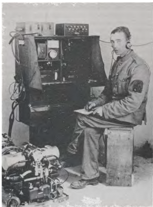
Portable wireless set powered by a twin-cylinder Douglas motor-bike engine, at Otranto 1917
