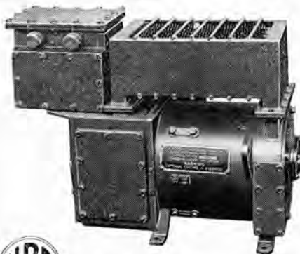
H.F. Motor Alternator for Radar. Output 2 KW. 80 volts A.C. 1,500 cycles per second. Watertight. Fitted with Automatic Voltage Regulator.
