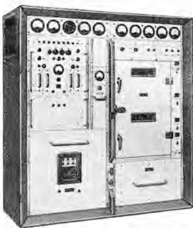
TA 184 10 kW linear amplifier
