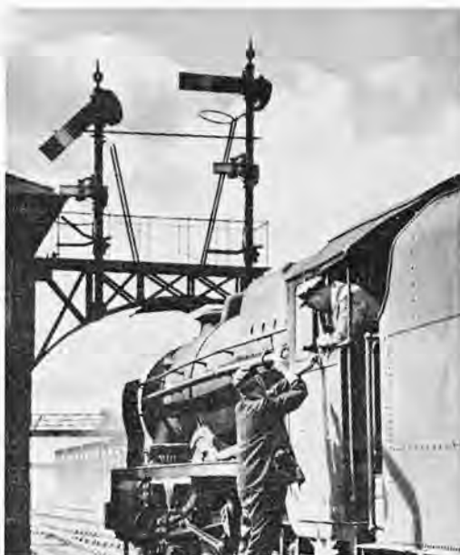
The two different positions of a 'lower quadrant' — 'home starter'. This indicates to the driver that he has the 'all clear' and proceed when ready. The through line however is blocked and no train must pass the horizontal semaphore.
