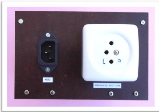
Figure 4 - Rear panel view showing inlet and outlet sockets
